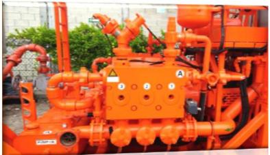
The design of the unit guarantees that the operators can monitor all the switches, instruments and the work conditions of all the systems in a conveniently and clearly way. There are Lights designed near of the instrument box and the displacement tank for night operations. The unit is equipped with 2 protection systems for guarantee the security of the equipment and the personal. One of them is the alvio safety valve and the digital overpressure.
